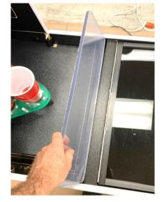
18) Remove the Protective Coating from the Side Shields. Using a 4 mm or 5/32" hex Allen-key to install the Side Shields using the screws provided in the Cash Box. Do not overtighten.
