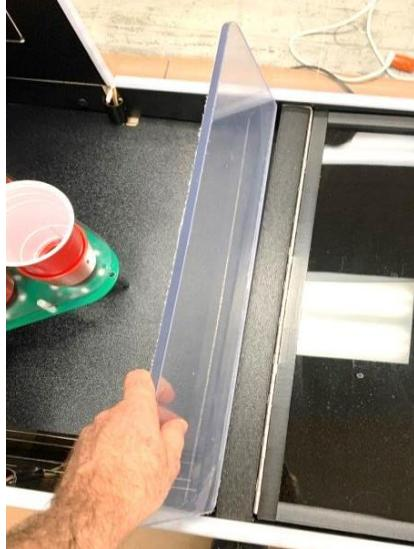
18) Remove the Protective Coating from the Side Shields. Using a 4 mm or 5/32" hex Allen-key to install the Side Shields using the screws provided in the Cash Box. Do not overtighten.
