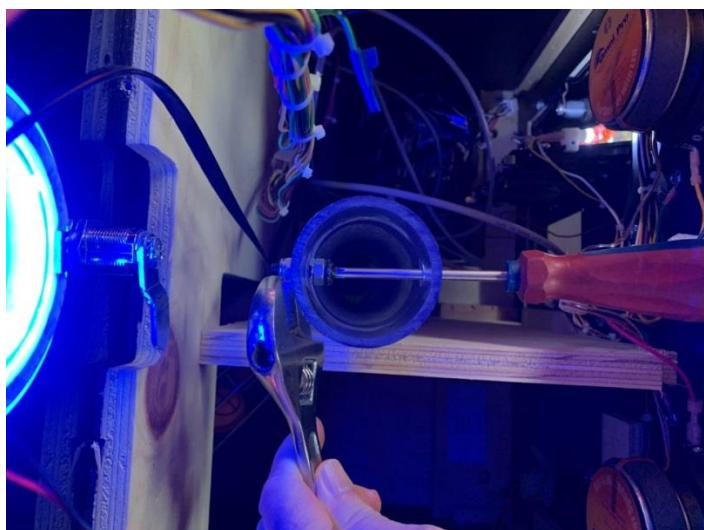
**2) Step 2:** Loosen Lock Nut on outside of chute.
