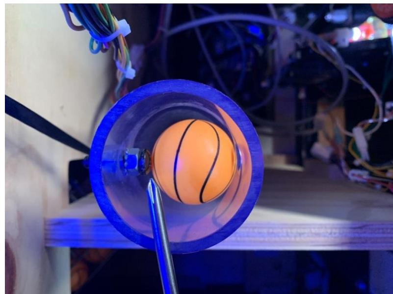
**5) Step 5:** If you want the ball to float higher simply adjust the 12 Vdc power supply screw in the cabinet to > 12.5 Vdc and < 13.0 Vdc. If you want the ball to float lower then adjust the 12 Vdc power supply screw in the cabinet to >12.0 Vdc and < 12.5 Vdc.
