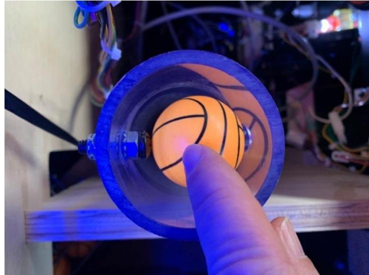
**4) Step 4:** Adjust the Speed Reducer screw so that the gap between it and the ball is minimal, almost rubbing. Launch a few balls to see how it behaves. Once it's launching properly tighten down the lock nuts on both sides of the chute wall. Try launching a few more balls to make sure.
